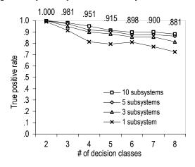
Fig. 4. Test set recognition ratio as a function of number of decision classes for different number of subsystems  $n_{\text{sub}}$ .
