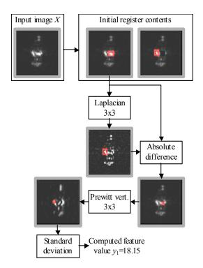
Fig. 5. An example of synthesized feature extraction procedure for BRDM image (azimuth 2.3°) as an input.
