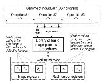
Fig. 2. Decoding and execution of LGP code contained in individual's I genome (for a single image X).
